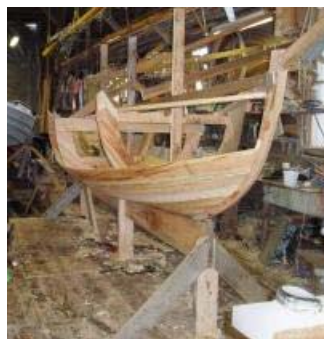
16' skiff under construction
